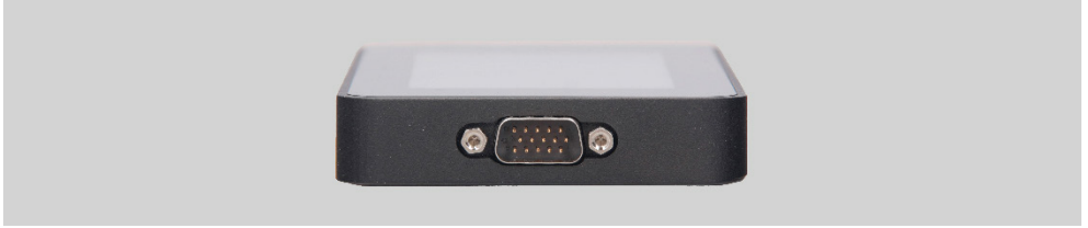
Figure 2. Terminal for connection of diagnostic cables
